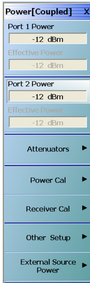
Figure 14-3. Main POWER Menu - Port 1 and Port 2 Coupled – Attenuators Installed
