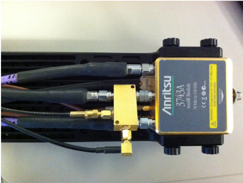
Figure 16-20. The connection of a Kelvin bias tee to a mm-wave module is shown here.
