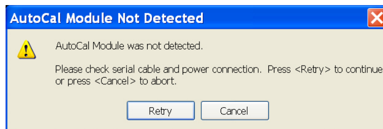
Figure 2-14. If the AutoCal module is connected incorrectly, the AUTOCAL MODULE NOT DETECTED warning message appears. Correct connections as required and click the Retry button.
